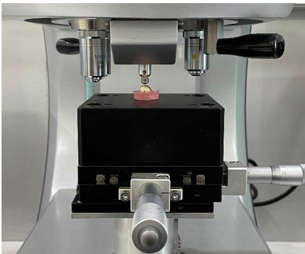
Figure 5: Shows the Vickers hardness test on the buccal surface of the tooth sample
