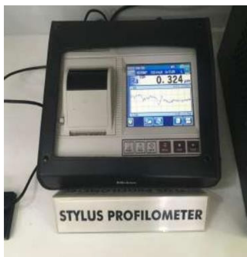
Figure 9: Roughness Average Calculated using the Stylus Profilometer
