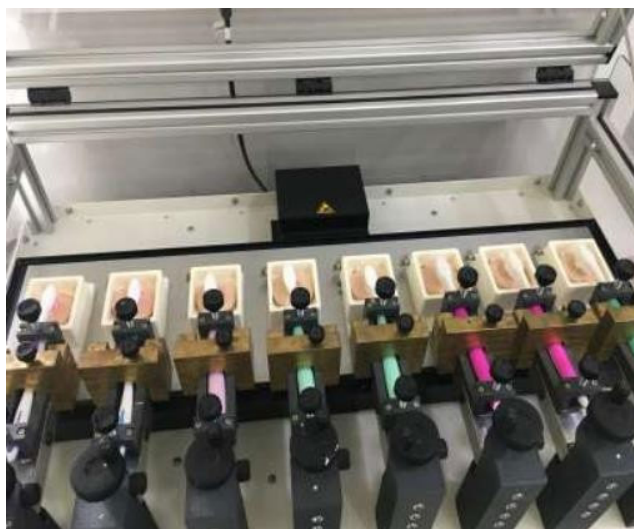
Figure 4: Sd Mechatronik Brushing Simulator Used For Brushing The Teeth Samples.
