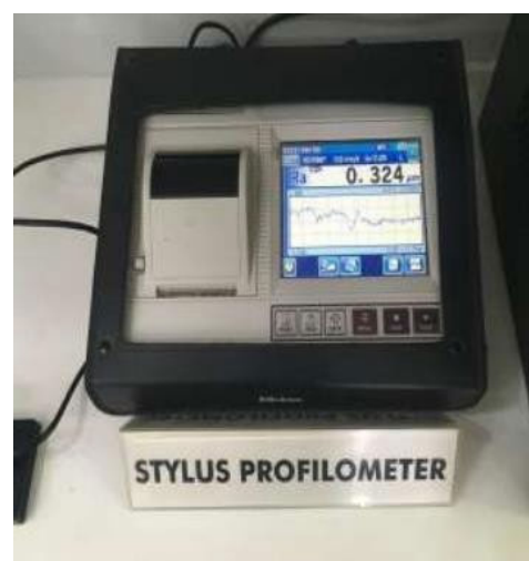
Figure 3: Roughness average calculated using the stylus profilometer
